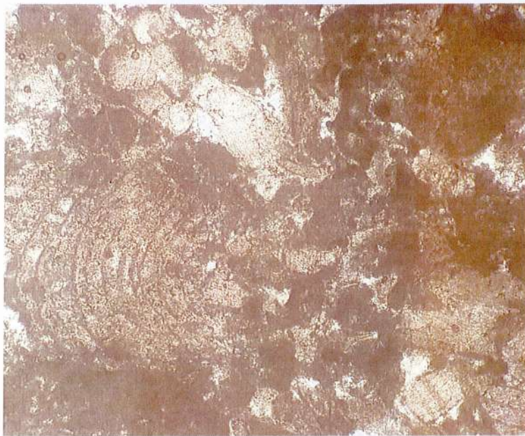
Figure 3: The sample under polarized light, magnified X times: red algae (left side)
