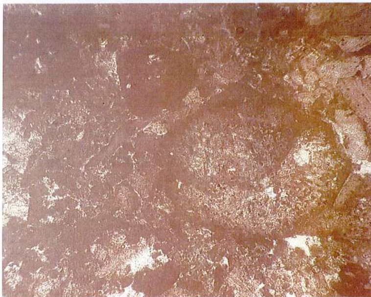
Figure 4: The sample under polarized light, magnified x times: Cayeuxia sp (cortoid) showing a thin micrite envelope
